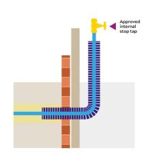
A BS 1010 internal stop tap must be installed as close as possible to where the pipework enters the property.
